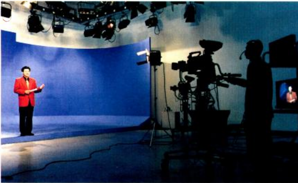
As shown here, the physical sets used with VR systems needn't be complex or large. In fact, one of the advantages of a VR set is that it can help create the illusion of space where there is little.
