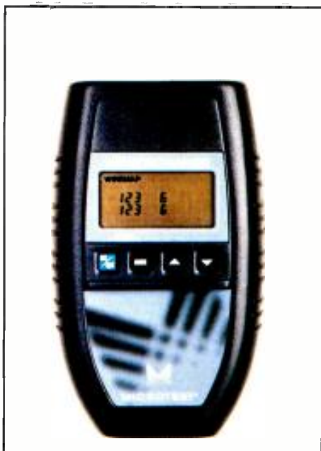
The Microtest MicroScanner is one of a variety of low-cost network testers.
